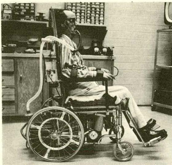
Figure 4. Ocular Controlled Wheelchair and Associated Equipment
