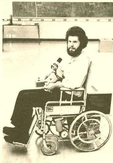
Fig 2. Photograph of Voice Controlled Wheelchair. Speech Recognition System is Mounted Behind Wheelchair
