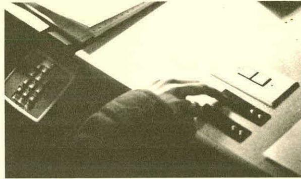
Having very limited strength and reach due to muscular dystrophy, he uses on-off and forward-reverse microswitches mounted into an adjustable table for easy reach. He manipulates the telephone push buttons with his thumb while supporting his hand on the table edge.
