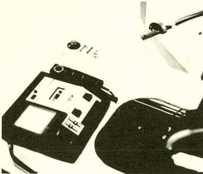
Figure 5: Dictator-Transcriber, shown on lapboard of wheelchair, is operated from breath tube top right.
